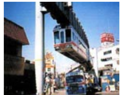
The French 'Safège' monorail, now built in Japan, floats along quietly on soft rubber tyres. Its supports need only to be the brilliant and powerful architecture of the Sixth Order.
