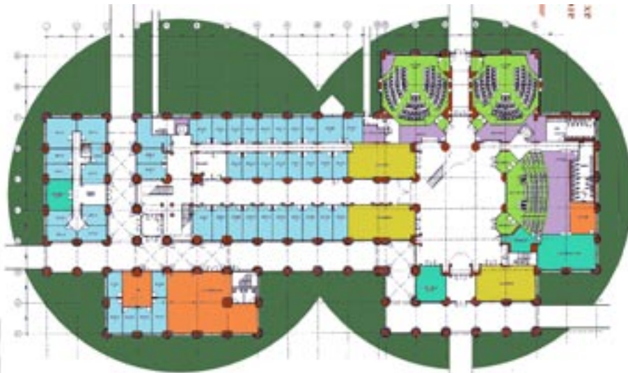
Plans of single and a 'double-bubble' 'Walking' columns. Note the four positions of walls around the yellow 'corridors'.
