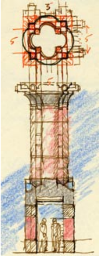
The Den Haag quatrefoil column and 'log and saddle' entablature, developed into its 'double-bubble form'.
